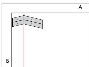
9. While aligning corners, insert the long tongue edge of plank #4 into the long groove edge of plank #2. Fully engage the long side joint by carefully tapping the edge using the prevail tapping block. Tap down the short joint with a lightweight soft-faced hammer.
