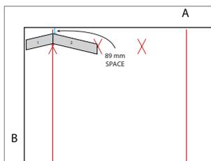
7. Align the short edge of plank #1 to the starting chalk line. Begin assembling the first V column with the point of the column 89 mm inches away from wall A. Precisely align and overlap the end joints of plank #1 and plank #2. Gently tap the top plank using a soft-faced hammer to fully lock the joints together.
