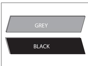
5. The chevron pattern planks are composed of two different shapes (mirror-images). These shapes are made easy to distinguish. One has a black pad, the other a grey pad. Separate grey pad and black pad planks from 3 or more cartons and mix to ensure a blend of pattern and shade. Black = A-plank / Grey = B-plank.
