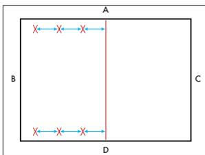
2. Begin at the center line near wall A, measure and mark in increments of 931 mm working toward wall B. Continue until no further increments can be marked. Repeat this process again near wall D.
