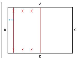
4. Measure and cut the starting planks equal to the distance from the starting line to wall B, allowing for the 3/8" (10mm) spacers. A T-Bevel (angle finder) can be used to find and mark the correct angle. Always measure twice before cutting. The material can be carefully cut using a variety of tools including: flooring shear, jig saw, circular saw, and table saw. (be certain to follow proper tool usage and safety procedures).
