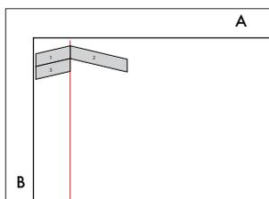
8. Cut the length of plank #3 for the second row. Insert the long tongue edge of the plank into the long groove of plank #1. Make sure there are no gaps. If necessary, carefully tap along the long groove edge of plank #3 using the prevail tapping block to close any gaps.
