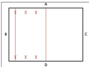
3. The final increment marks nearest wall B will be used to create the starting line. Snap a chalk line connecting the last two marks. This line will indicate the center of the first V column. Note - Aesthetically, if the width of the first column is too narrow the starting line may be offset toward the center line by 465 mm.
