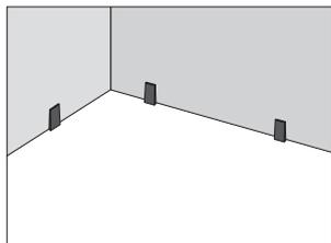
6. Create the required expansion by placing 3/8" (10mm) spacers between the flooring assembly and the walls.
